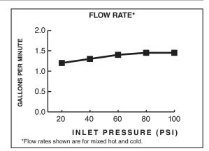
1.5 gpm/5.7 L/min. FLOW RATE
